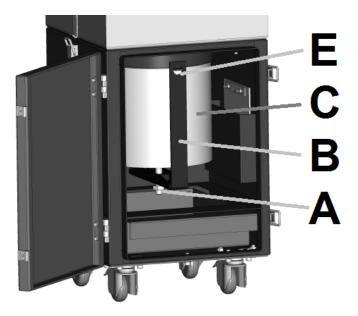
Before changing the filter cartridges hold ready an appropriate container (e.g. PE bag) for disposal.
